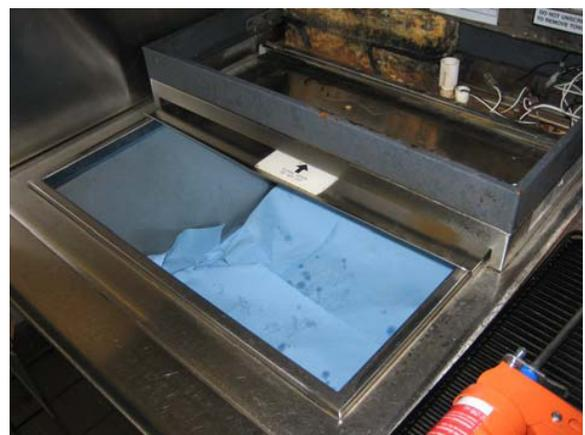
7. If mold is present, spray the mold areas with the Kay 5 solution or Tilex and let sit for 30 - 60 seconds.
