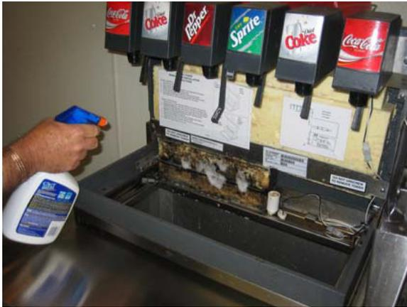
8. Clean/brush the mold area by brushing the cleaning solution over the mold area (Recommended brush has a smaller head to fit into the tighter areas).
