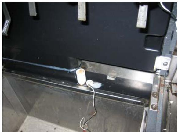
34. Install the drain coupler/seal on the drain tube (Lancer units only)
