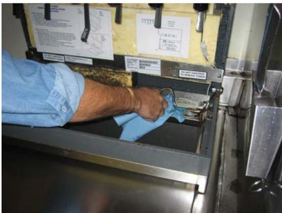
12. Using the heat blower, dry the insulation. Typically drying takes 3 to 5 minutes. Move the blower around to prevent excessive heating of the foam.
