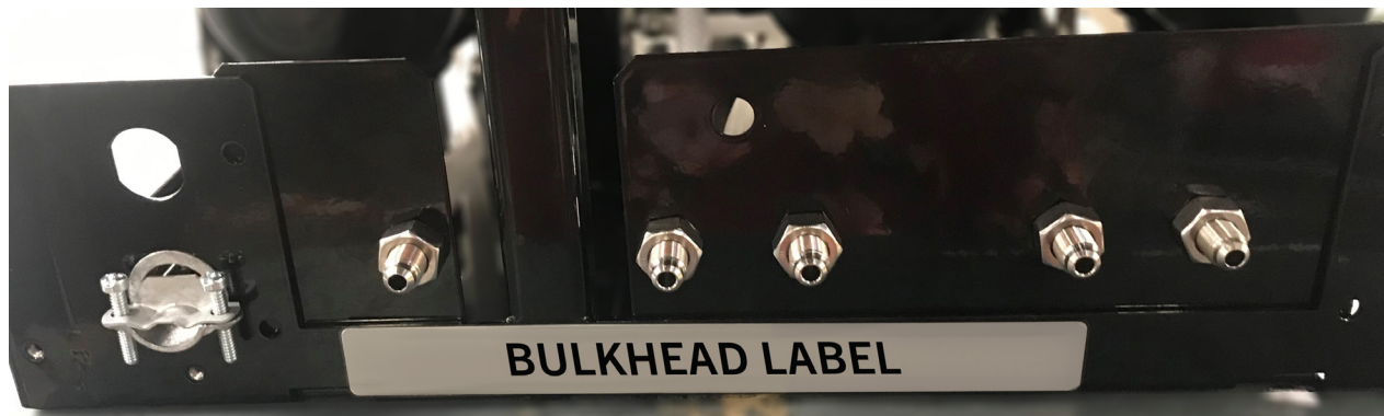
Figure 4.3 Bulkhead Fittings Label Location
