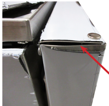
Minor door damage close-up
