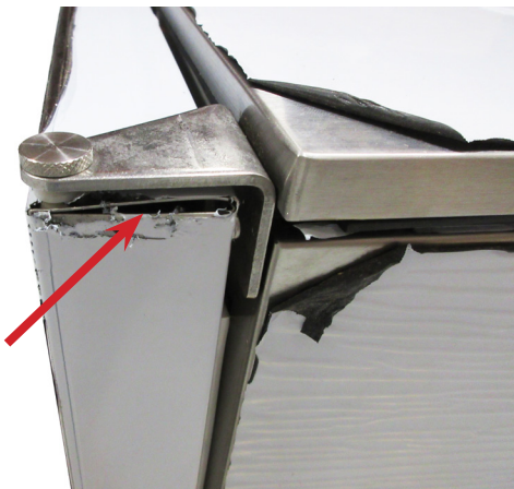
Minor door damage close-up
