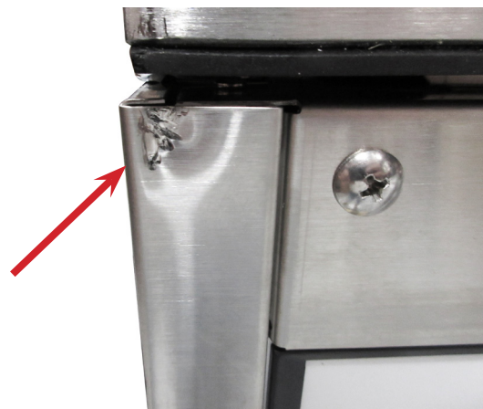
Minor door frame damage close-up
